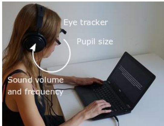
Figure 1. Augmented interoception by mapping pupil size that is recorded with an eye-tracker in real-time, to changes in the volume and frequency of an audible sound (sine wave). This setup was used in study 2 that was discussed.
