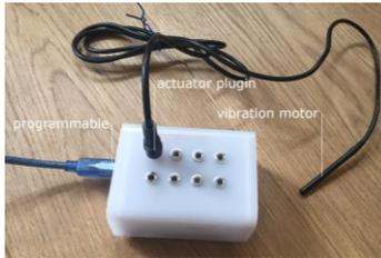
**Figure 4:** A new version of the tactile vision interface, with vibration motors
