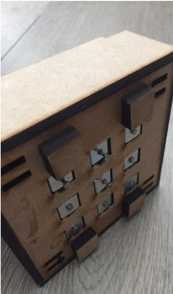
**Figure 2:** Back of the haptic vision interface, with solenoids.
